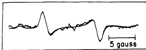
Figure 6. Computer-simulated Pake-doublet spectrum (smooth curve) superimposed on an experimental proton spectrum of potassium oxalate monohydrate (after ref 118).
